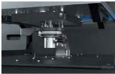
Interchangeable platens with enhanced height adjustment and optical sensing
